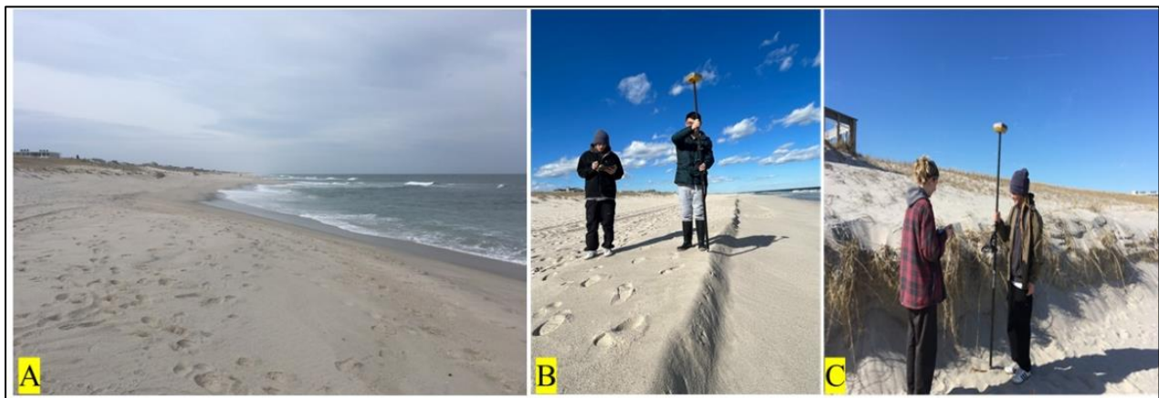
Fig.5 field photos A) was taken on March 17 at the survey line 3, looking towards the line 4. The beach was much wider at line 3 and abruptly became narrow at line 4. B) was also taken on March 17 at profile 4, where a beach scarp formed. C) an existing dune scarp measured on Feb 10, 2023.
